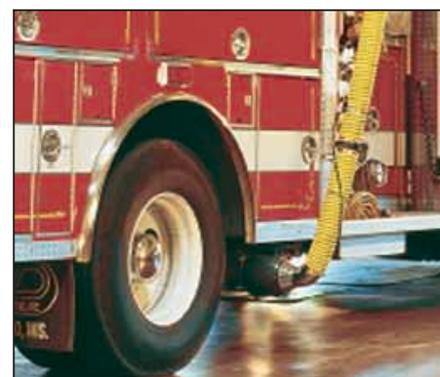
*PlymoVent was the pioneer of the inflatable tailpipe nozzle, which is today the standard of the industry. It's leakproof design guarantees no escape of exhaust gases from around your tailpipe.*
