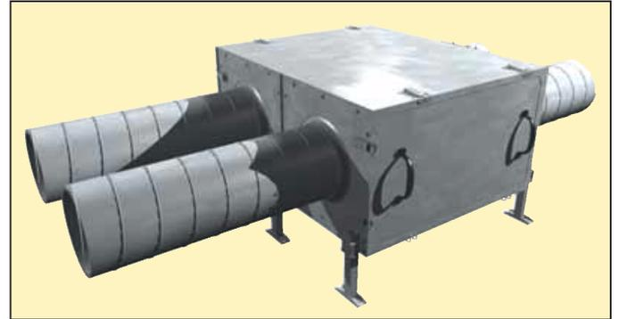
The negative pressure design uni-filters are equipped with 400 mm/16" diameter inlet and outlet that can be reduced for smaller duct work diameters and lower air volumes. The uni-filter can be placed before the fan and anywhere after the last point of extraction or hose drop.
