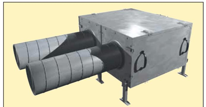
The positive pressure design uni-filters are equipped with a 400 mm/16" inlet and a flat louver outlet grille. The inlet can be reduced for smaller duct diameters or air volumes and the outlet grille can be rotated in four directions of discharge.
